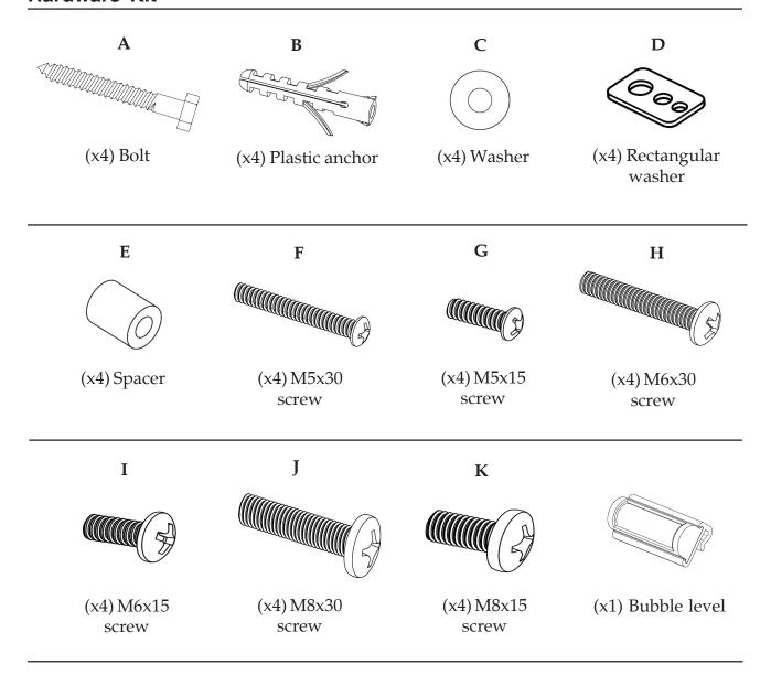
**Important**: The Low Profile Universal TV Mount - 32" to 65" is shipped with the proper installation hardware and parts. Make sure that none of the items are missing or damaged before starting the installation. If there are any missing and/or damaged parts, please stop the installation and contact your place of purchase.
